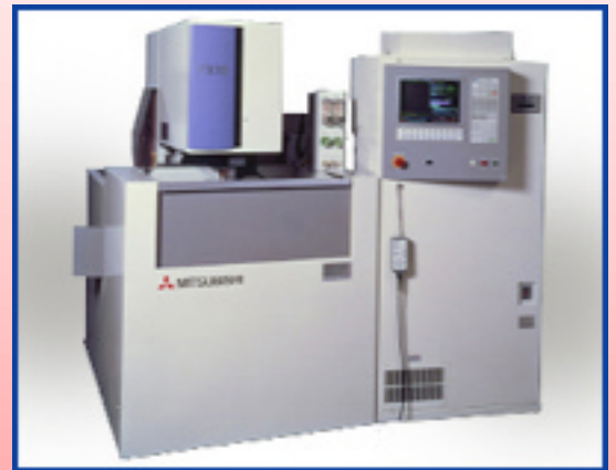
MITSUBISHI FX 10K WIRE EDM (WITH AUTOTHREADING FOR UNATTENDED OPERATION) 31.5"x22.6"x8.5" (WxDxH)
